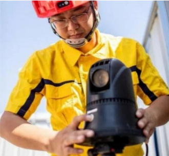
• "Dome Camera + Smart Helmet" for back-office supervision of engineering construction in real time
